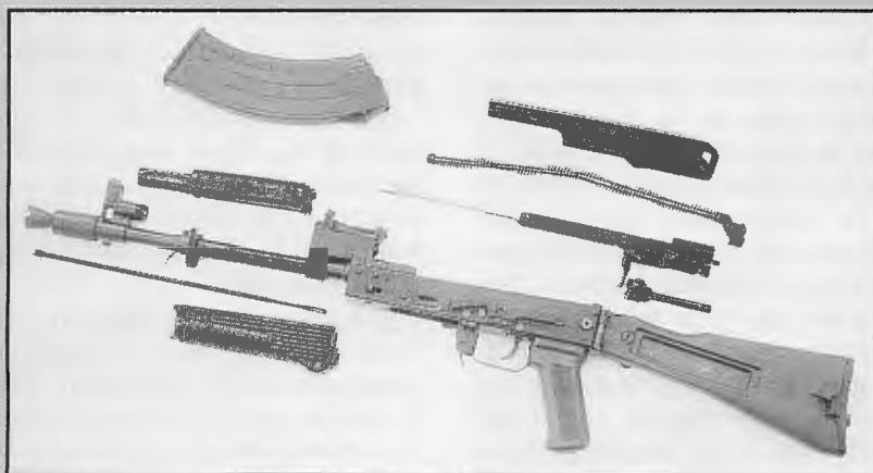
Caliber 7.62x39mm AK104, fieldstripped.
